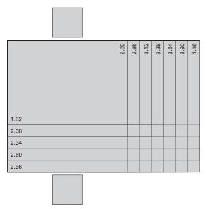
Car width and length can be extended in steps of 65 mm, 130 mm or 260 mm.
