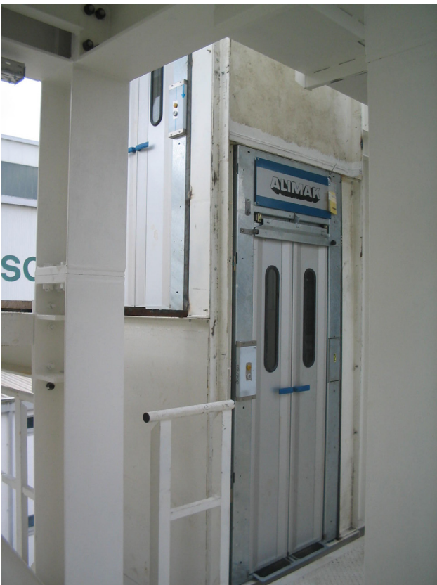
Alimak elevator inside the world's largest tunnel boring machine.
